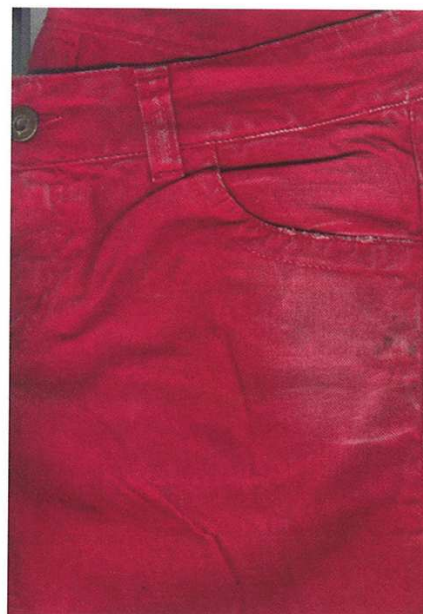
With the CDS no dyeing auxiliaries are needed to get bright coloured denim garments that have an indigo-dyed look.
